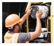
RADIAL SEAL ENGINE AIR FILTER
